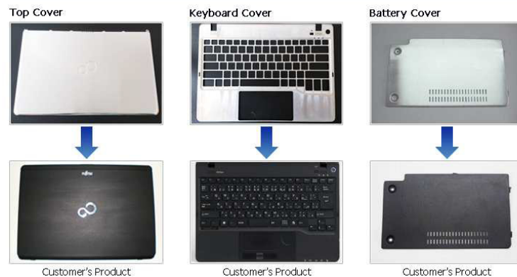
Mass Production Press Forming of a Magnesium Alloy (AZ31) for a Variety of Products
